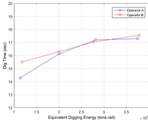
**Figure 11.** Average dig time for different digging energy classes.
