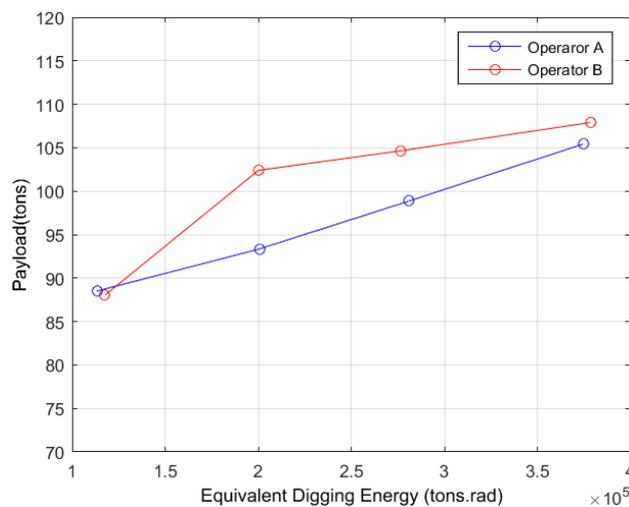
**Figure 12.** Average payload for different digging energy classes.
