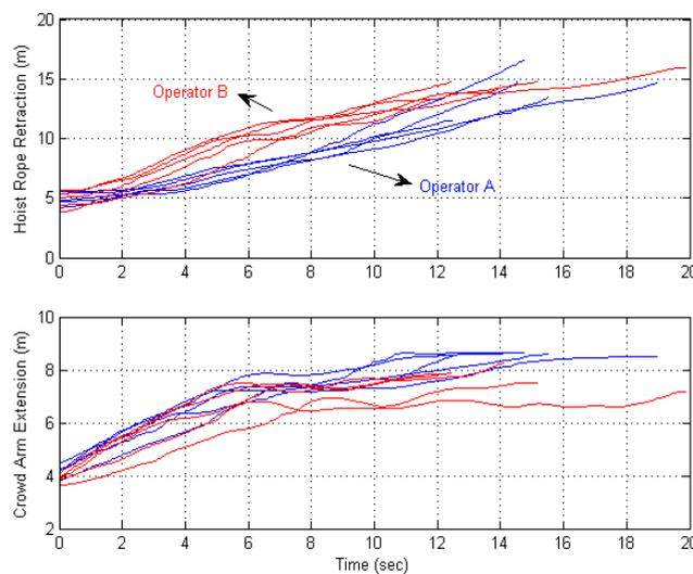
**Figure 14.** Hoist rope retraction and crowd arm extension for Operators A and B.
