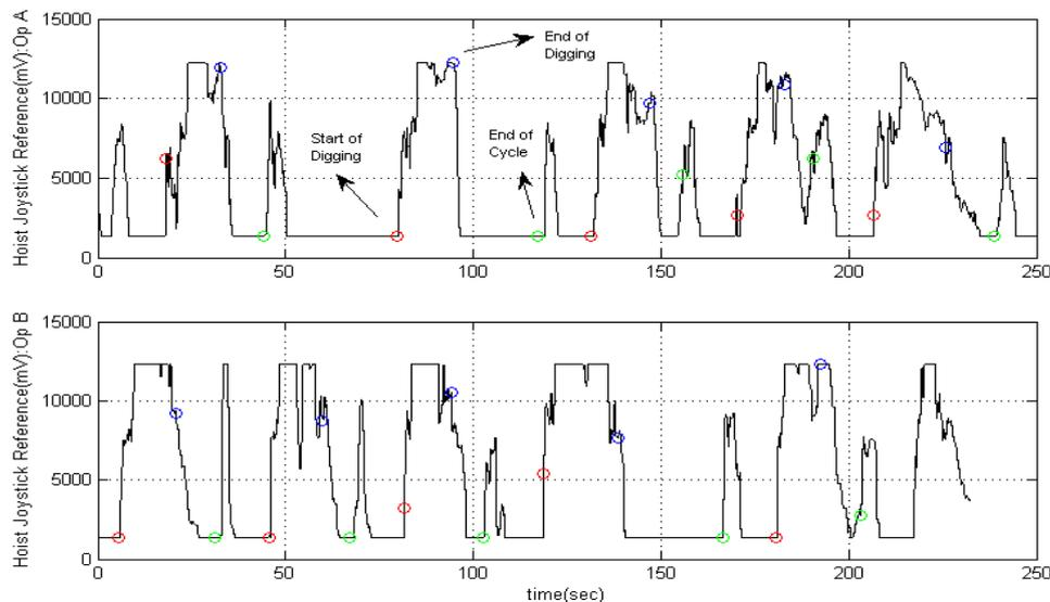
Figure 9. Hoist joystick reference.
