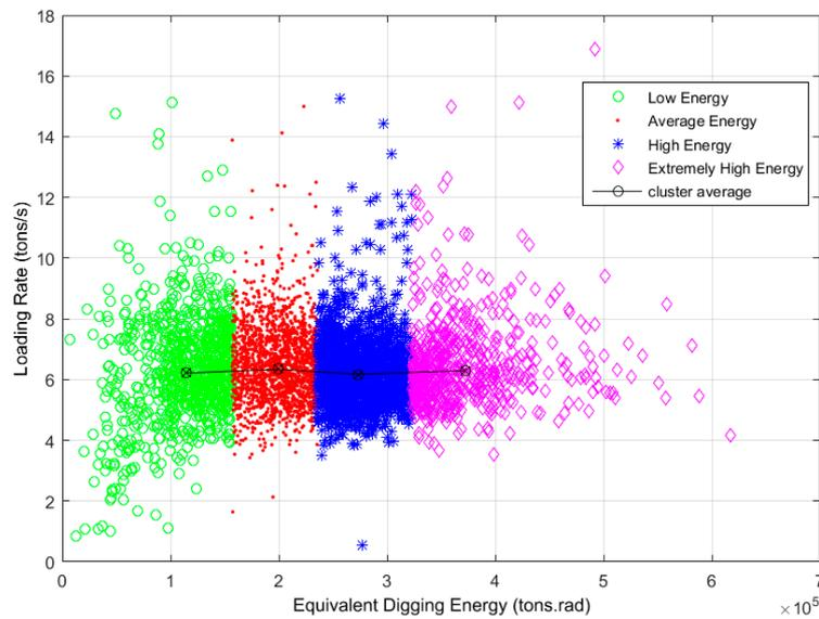
Figure 7. Loading rate vs. digging energy for all operators.
