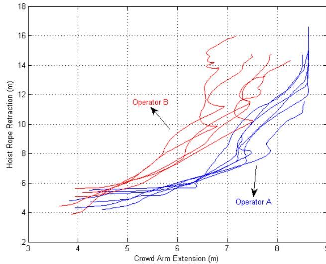
**Figure 13.** Digging trajectory for Operators A and B
