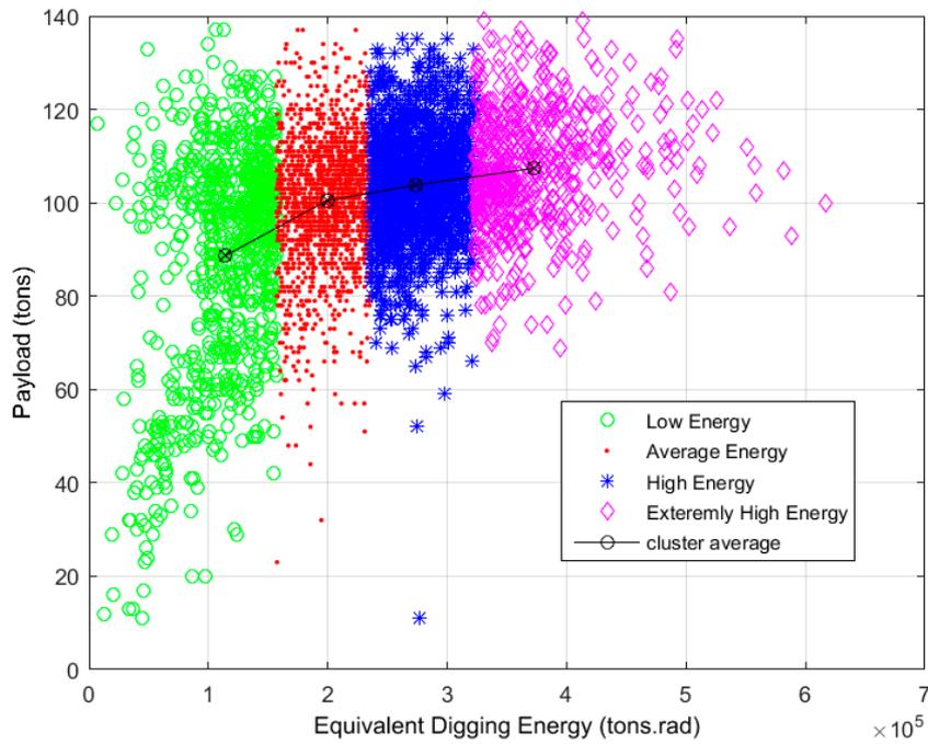
Figure 5. Result of clustering analysis for comparison of payload and equivalent digging energy.
