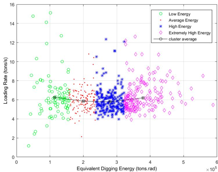
Figure 8. Loading rate vs. digging energy for Operator A.
