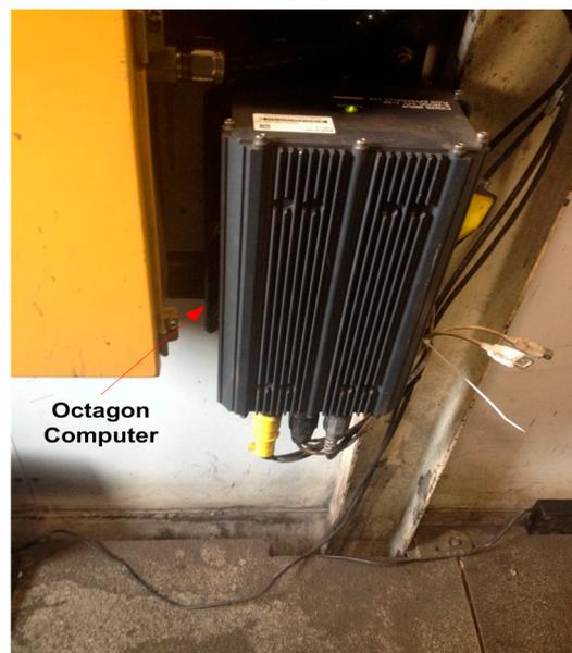
Figure 1. Octagon computer installed in the shovel house.
