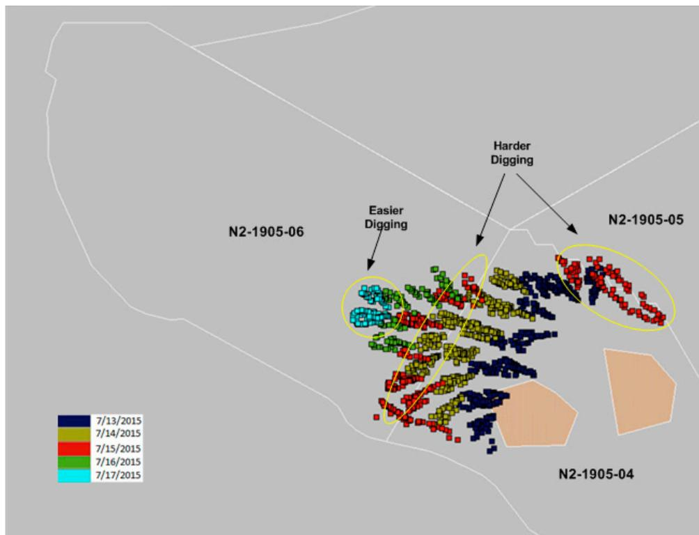
**Figure 2.** Shovel dig playback during the field trial (provided by mine).
