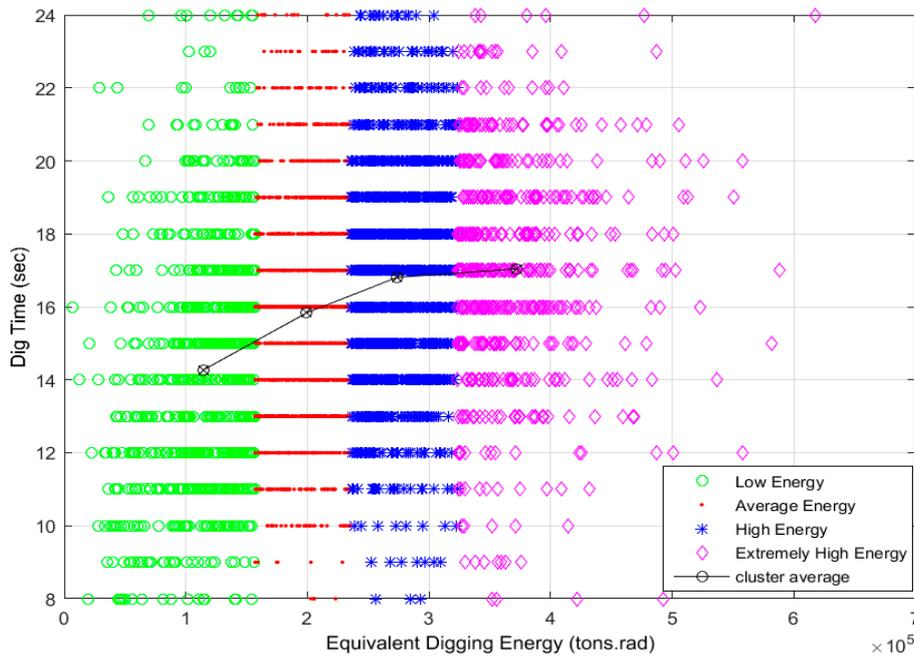
Figure 6. Result of clustering analysis for comparison of dig time and equivalent digging energy.
