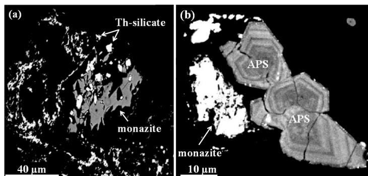
**Figure 1.** Examples of intensive alteration of monazite by diagenetic/hydrothermal brines from the basement of the Proterozoic Athabasca Basin (Canada): (a) Back-scattered electron image of a monazite grain (grey), which is nearly completely altered to Th-silicate (white) (modified from [17]). (b) Back-scattered electron image of a relict monazite (white) associated with aluminum phosphate-sulfate mineral (APS) (grey) (modified from [57]).
