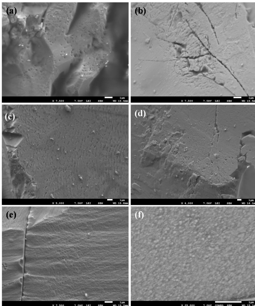
**Figure 4.** SEM images of the different alteration features on monazite grains after the six months experiments: (a) etch pits in EXP# 20; (b) etch pits and roughened surface in EXP# 13; (c) etch pits and roughened surface in EXP# 22; (d) etch pits and roughened surface in EXP# 16; (e) roughened surface in EXP# 17; and (f) zoom into roughened surface in EXP# 17.
