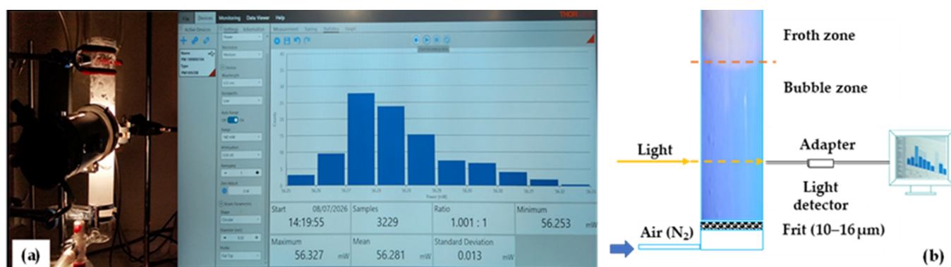
Figure 1. Experimental setup for bubble coalescence measurements (a) Photograph of the experimental setup (b) Schematic representation of the experimental setup [36].
