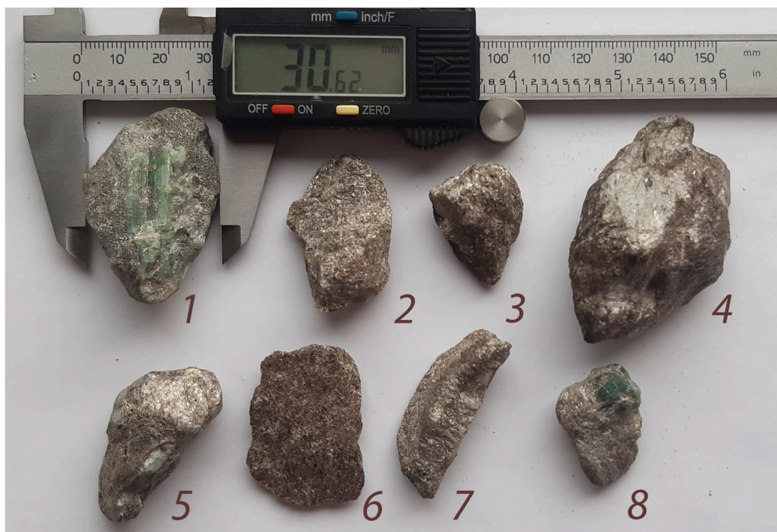
Figure 4. Photographs of the mineral samples used in the experiments. Beryl crystals with a greenish tint are visible on samples 1, 4, 5, and 8; sample 6 is muscovite without inclusions; in the remaining samples, the beryl is hidden.
