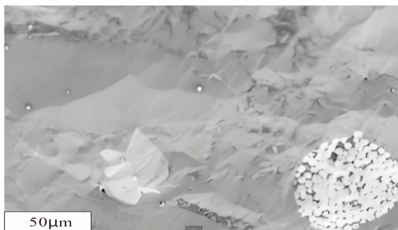
Figure 11. Scanning Electron Microscope (SEM) image of argillaceous shale from Well Y104 (2992.16 m).
