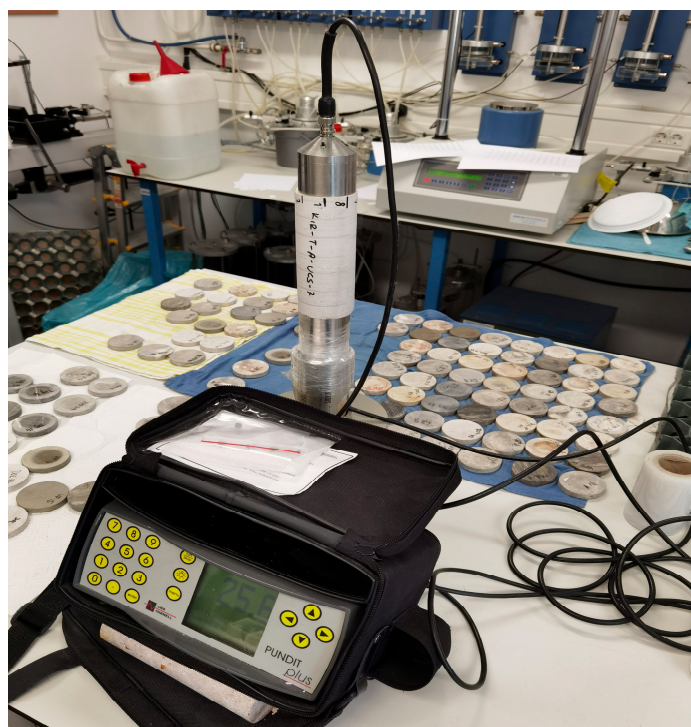
Figure 2. Measuring of the ultrasonic wave velocity through the sample.
