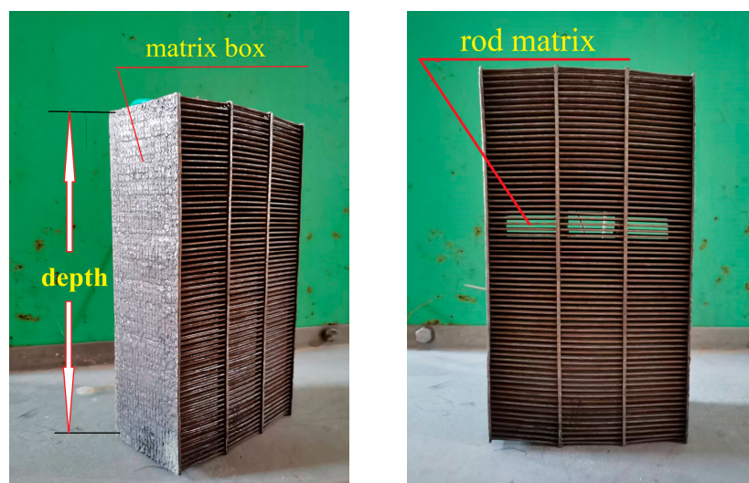
Figure 12. Typical matrix box in a pilot-scale transverse-field HGMS with a diameter of 2 mm.
