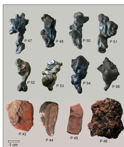
Figure 10. Selected analyzed samples of archaeological slags (upper two rows) and ores (lower row) from the Sehnde 9 site.
