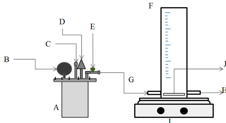
**Figure 2.** Bench-scale flotation system: (A) saturator vessel; (B) manometer; (C) pressurized air inlet; (D) pressure relief valve; (E) needle valve; (F) flotation column; (G) DAF microbubbles inlet for air-saturated liquid; (H) outlet for sample collection for analysis; (I) magnetic stirrer; (J) magnetic stir bar.
