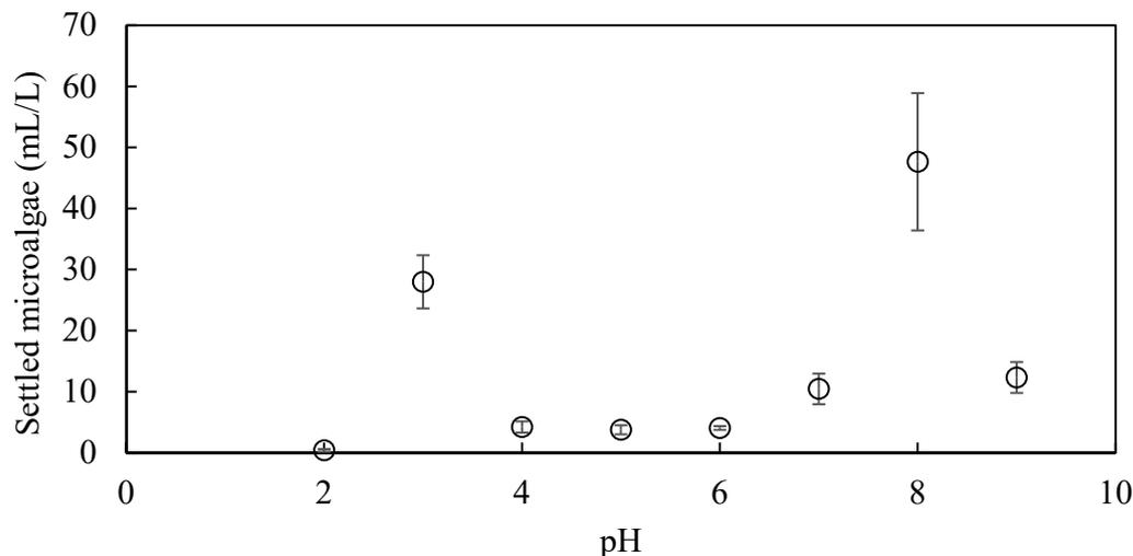
**Figure 4.** The volume of *Scenedesmus* sp. cells settled in the Imhoff cone as a function of pH.
