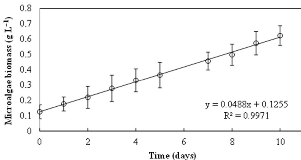
**Figure 3.** Evolution of biomass concentration during the cultivation of microalgae in acid mine drainage supplemented with nutrients.
