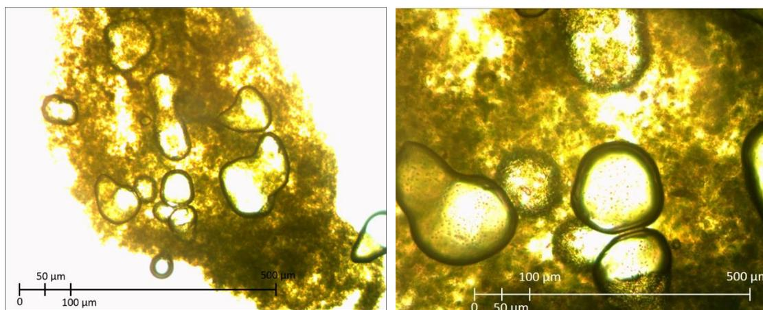
**Figure 8.** Aerated floc of microalgae with multiple bubbles, captured during ascension in the DAF column. Conditions:  $0.3 \text{ mL L}^{-1}$  Tanfloc SG;  $2 \text{ mg L}^{-1}$  anionic polyacrylamide;  $\text{pH} = 8 \pm 0.1$ ; a saturation pressure of 5 atm; and a recycling ratio of 20%. Visualised under optical microscopy at  $100\times$  magnification.
