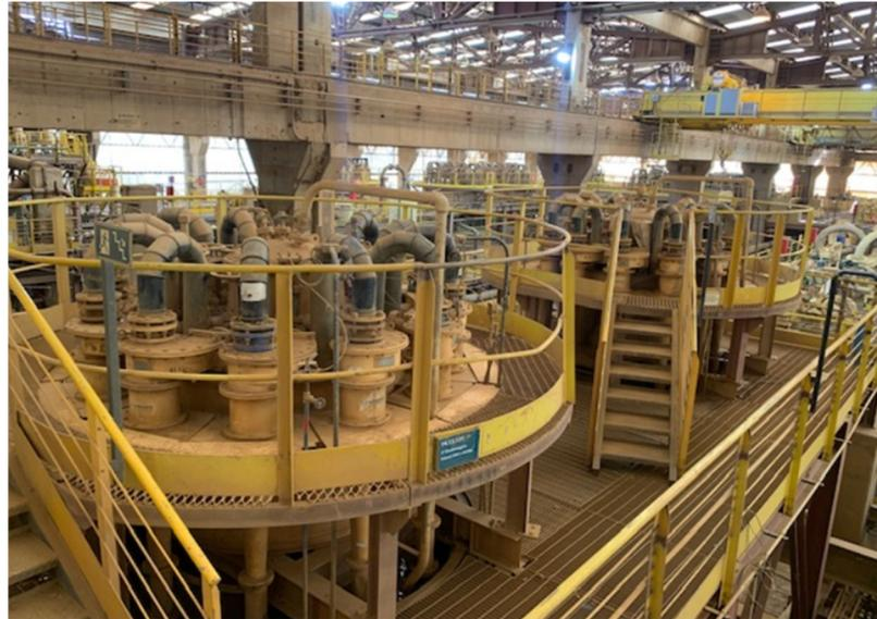
**Figure 3.** Tapira industrial circuit—second desliming stage.
