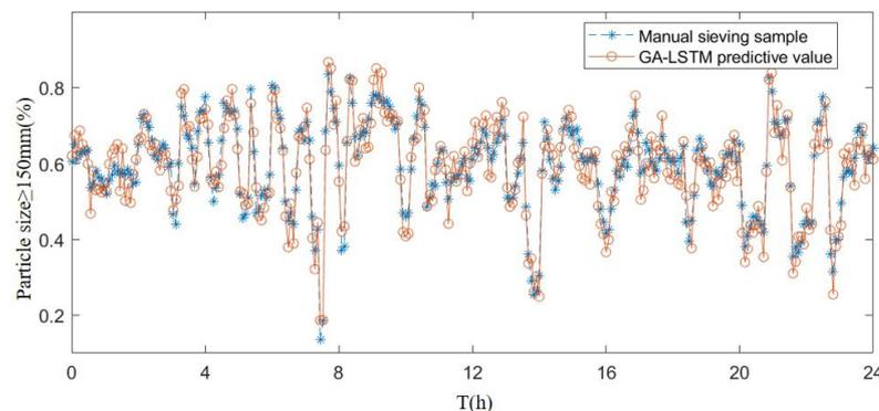
Figure 6. Lump size prediction of SAG mill feed.
