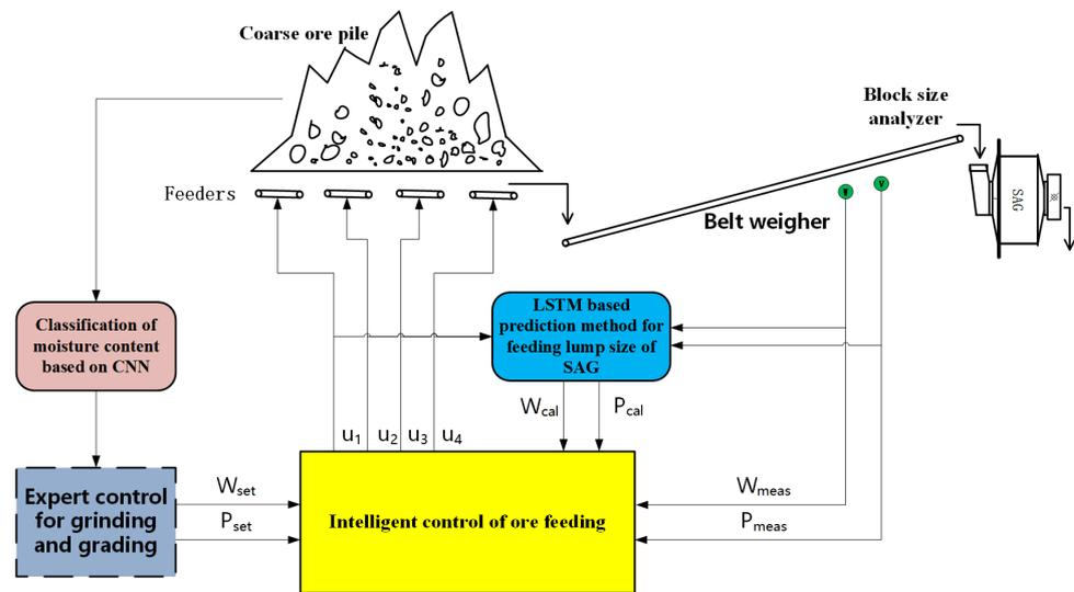
Figure 9. Intelligent control of ore-feeding plus compensation module.
