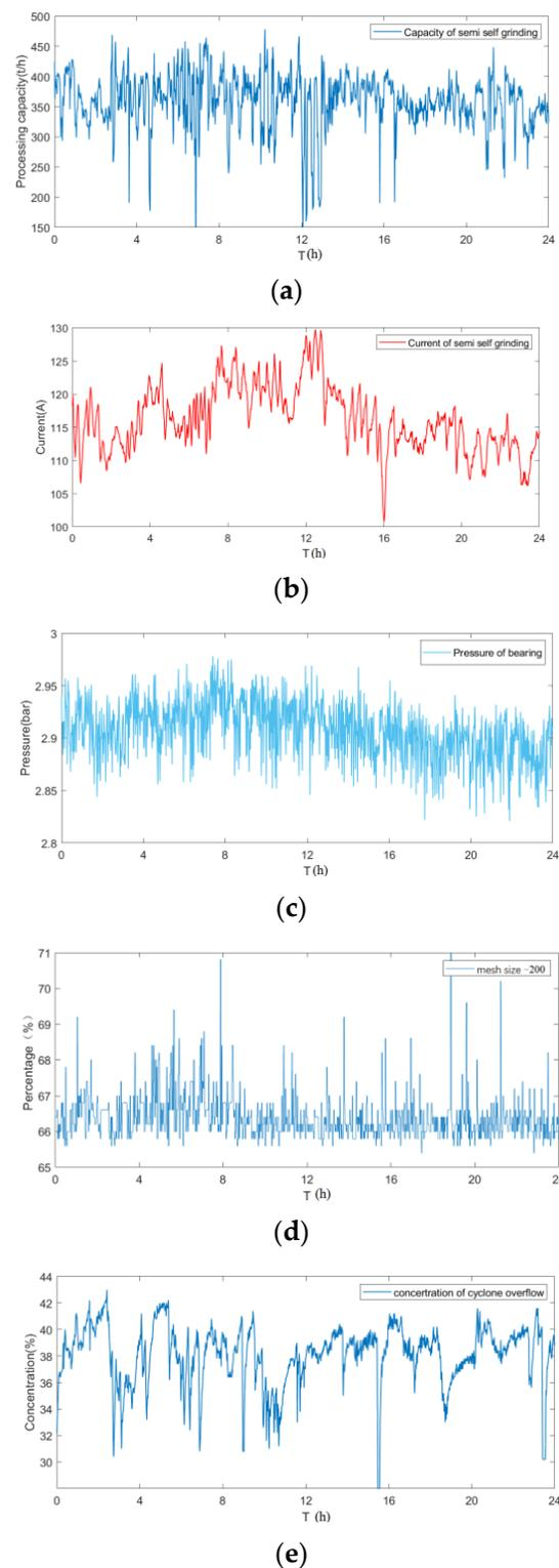
**Figure 2.** Difficulty in stabilizing the industrial grinding process. (a) Throughput of SAG Mill. (b) Current of SAG mill. (c) Pressure of bearing. (d) Percentage of mesh size ( $-200$ ). (e) Concentration of cyclone overflow.
