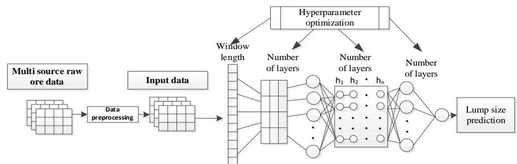
**Figure 4.** Prediction of grinding fragmentation based on LSTM.
