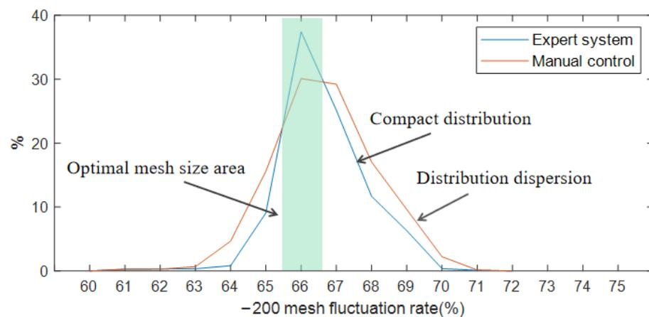
Figure 12. Particle size distribution statistics of grinding products.
