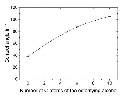
**Figure 3.** Contact angles of pristine glass slides (C0) and those esterified with 1-Hexanol (C6) and 1-Decanol (C10) measured in sessile drop mode via optical contour analysis against water. The glass slides have the same chemical composition as do the glass particles used in this study and their esterification is conducted in the same way as that of the glass particles. The error bars represent the 95% confidence interval. Lines are added to guide the eyes.
