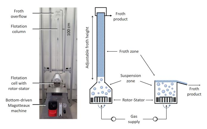
**Figure 4.** The *MultiDimFlot* separation apparatus in the lab (**left**), schematic drawings of *MultiDimFlot* (**middle**) and the conventional agitator-type froth flotation cell (**right**) used for the flotation tests in this comparative study.
