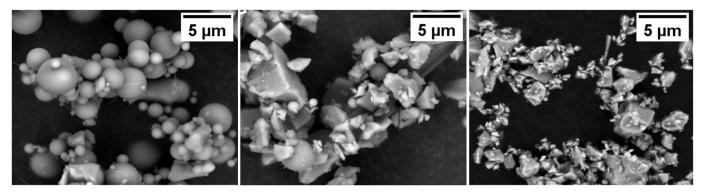
**Figure 1.** Scanning electron micrographic images of glass spheres (**left**), glass fragments (**middle**) and magnetite (**right**).
