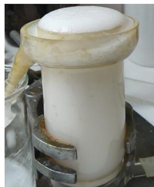
**Figure 18.** Photos of flotation of 1 wt.% KERMA 90-45 of 0.05 mol/L hexylamine with flotation yield = 18.3% ( $\zeta_1 = 65$  mV,  $\zeta_2 = -6$  mV).
