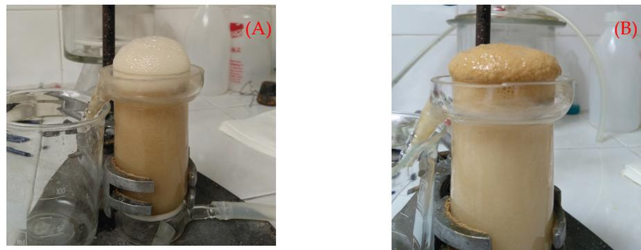
**Figure 16.** Photos of flotation of 1 wt.% STERILES-MS 45 in the presence of (A)  $10^{-4}$  mol/L MIBC with flotation yield = 7% ( $\zeta_1 = -65$  mV,  $\zeta_2 = -13.3$  mV), and (B) 0.05 mol/L hexylamine with flotation yield = 61% ( $\zeta_1 = 65$  mV,  $\zeta_2 = -18.6$  mV).
