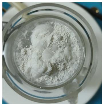
**Figure 21.** A photo of hydrophobized with hexamethyldisilazane silica in the flotation cell.
