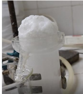
**Figure 22.** Photo of flotation froth containing pure magnesite ( $\text{MgCO}_3$ ) with collector  $3 \times 10^{-3}$  mol/L disodium dodecyl phosphate and in the presence of  $5 \times 10^{-4}$  mol/L (50 ppm) MIBC.
