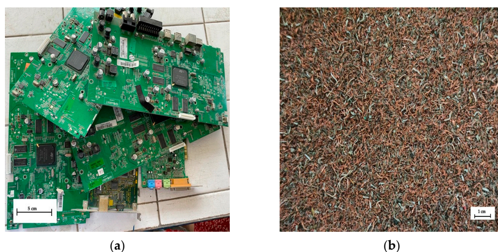
Figure 1. The samples used in experimental studies: (a) EOL PCBs and (b) WEWs.
