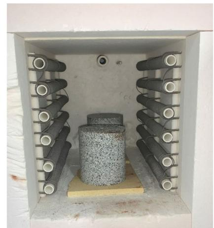
**Figure 7.** (a) Heating history graph of the Tashmurunsky granite thermal treatment process; (b) high-accuracy, electric, fiber-insulated chamber furnace SNOL 30/1300.
