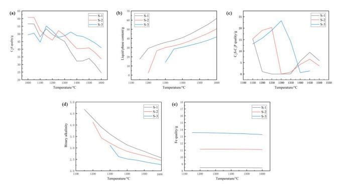
**Figure 3.** Equilibrium phase composition of tempered slag (( $\mathbf{a}$ - $\mathbf{e}$ ) represent C<sub>2</sub>S mass fraction, liquid mass fraction, C<sub>2</sub>S-C<sub>3</sub>P mass fraction, basicity, and Fe content, respectively).
