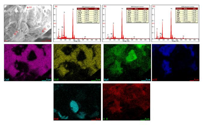
**Figure 5.** SEM morphology, face scan, and energy spectrum in S-1 (In the figure, "+" represents the position of the point, and "a-c" represents the corresponding sequence number).
