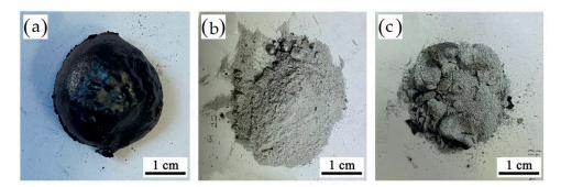
**Figure 1.** Tempered slag roasted specimens ((**a**–**c**) mixed with 3%, 4%, 5% SiC reagent slag, defined as S-1, S-2 and S-3).
