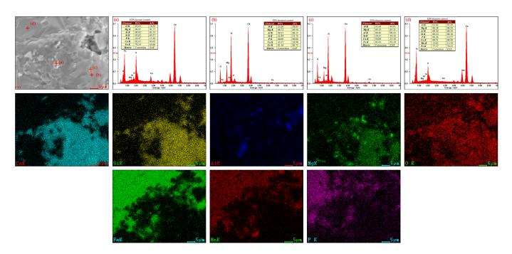
**Figure 6.** SEM morphology, face scan, and energy spectrum in S-2 (In the figure, "+" represents the position of the point, and "a–d" represents the corresponding sequence number).
