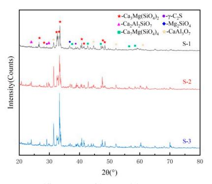
$\label{lem:Figure 4.} \textbf{XRD diffraction pattern of the tempered-slag specimen}.$
