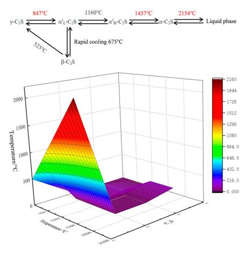
**Figure 2.**  $C_2S$  crystal shape transition with temperature (different colors indicate different temperature ranges).
