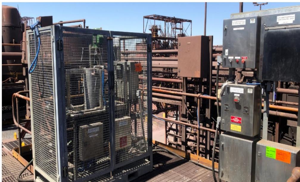
**Figure 1.** An installed PCM® at BHP Olympic Dam. The PCM® is installed on the rougher flotation circuit of the concentrator.
