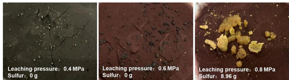
Figure 13. Images of the pressure leaching products at different oxygen pressure.
