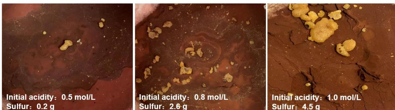
Figure 4. Images of the pressure leaching products with different initial acidity.
