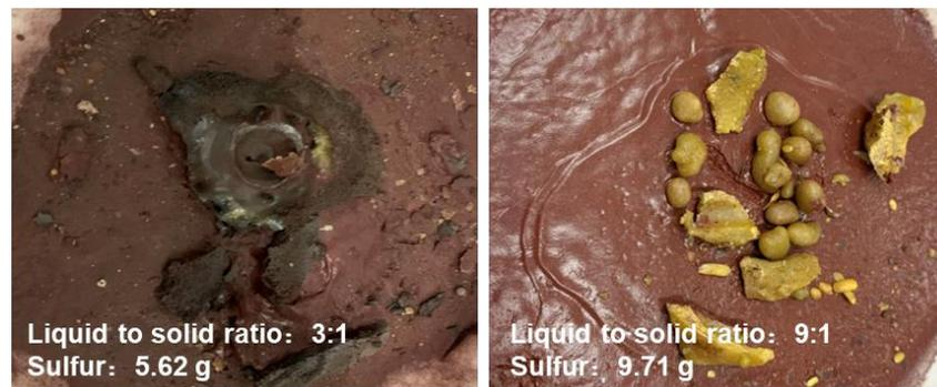
Figure 16. Images of the pressure leaching products with different liquid-to-solid ratios.
