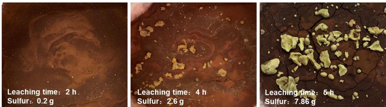
Figure 7. Images of the pressure leaching products with different leaching times.
