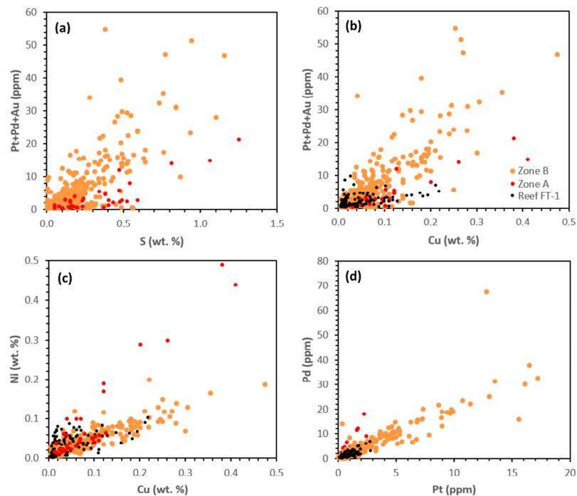
**Figure 12.** Binary diagrams S vs. Pt + Pd + Au (a), S vs. Pt + Pd + Au (b), Cu vs. Ni (c) and Pt vs. Pd (d) for the mineralized rocks of the PGE zone B (402 samples, East Chuavry deposit) compared with other PGE zones of the East Pana intrusion and the FT-1 reef in the Fedorova intrusion. Analytical data for core samples from [50,59], two grab samples of the FT-1 reef from [13]. Pt + Pd + Au > 0.5 ppm.
