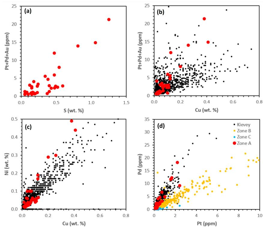
**Figure 11.** Binary diagrams S vs. Pt + Pd + Au (a), S vs. Pt + Pd + Au (b), Cu vs. Ni (c) and Pt vs. Pd (d) for the mineralized rocks of the PGE zone A (35 samples, representative drill holes P-253 and P-350 of the Churozero and Chuavry sites, respectively) compared with other PGE zones of the East Pana intrusion and the Kievey deposit in the North PGE reef of the West Pana intrusion. Analytical data for core samples from [42,50], Pt + Pd + Au > 0.5 ppm.
