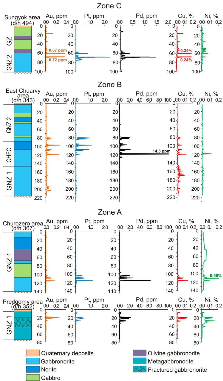
**Figure 14.** Stratigraphic columns for representative drill holes in the PGE zones of the East Pana intrusion with variations of Au, Pt, Pd, Cu and Ni.
