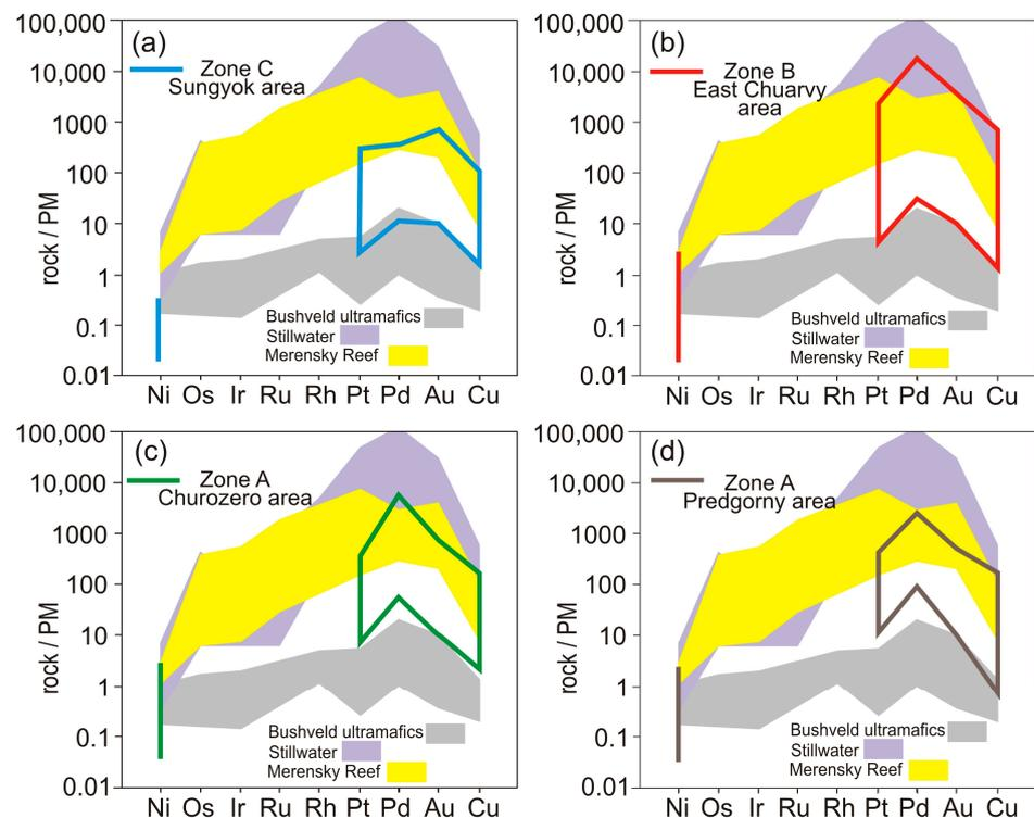
**Figure 15.** Primitive mantle–normalized chalcophile element patterns in the PGE zones of the East Pana massif (PGE zone B,C—(a,b), PGE zone A—(c,d)) compared to the Bushveld Complex [62] and Stillwater Complex [11]. Normalization factors from Barnes and Maier [62].
