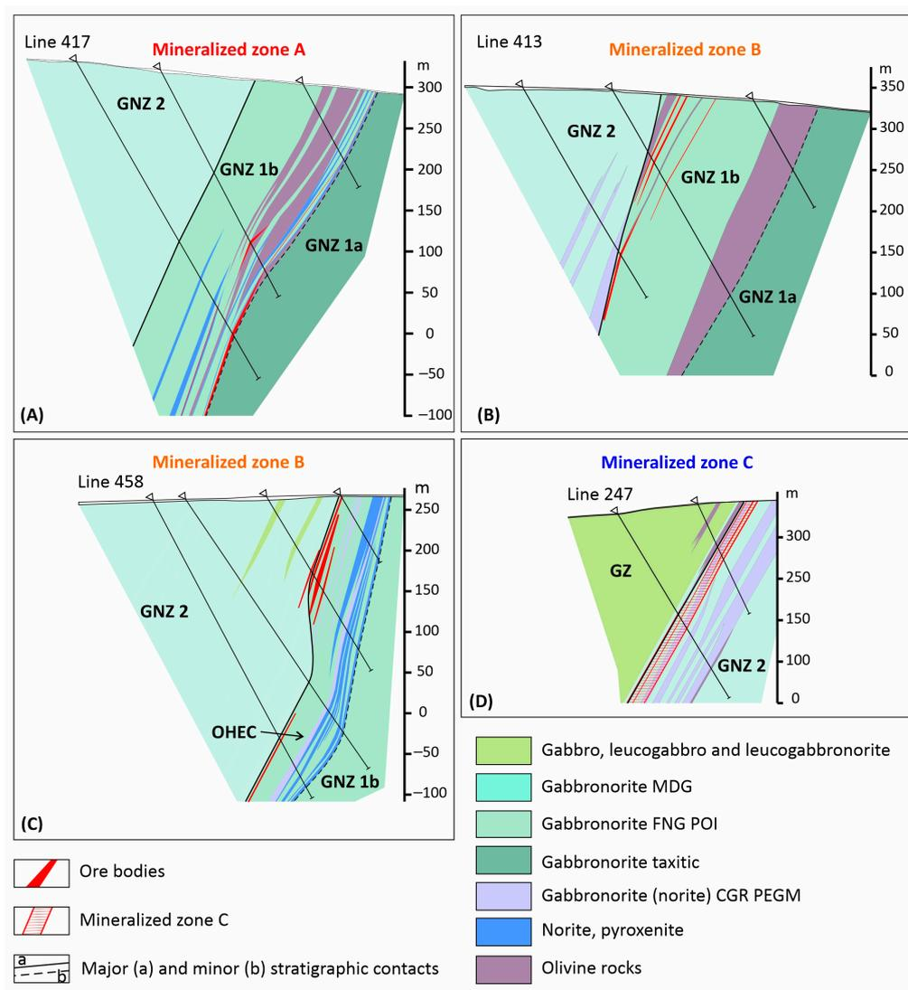
**Figure 2.** Schematic geological sections through the PGE zones of the East Pana intrusion: PGE zone A (A), PGE zone B (B,C), PGE zone C (D). GNZ, gabbronorite zone; GZ, gabbro zone, OHEC, Ore Horizon of the East Chuarvy deposit; FNG, fine-grained; MDG, medium-grained; CGR PEGM, coarse-grained to pegmatoid; POI, poikilitic. Lines of geological profiles and their location within the areas are shown in Figure 1. Modified after [50].
