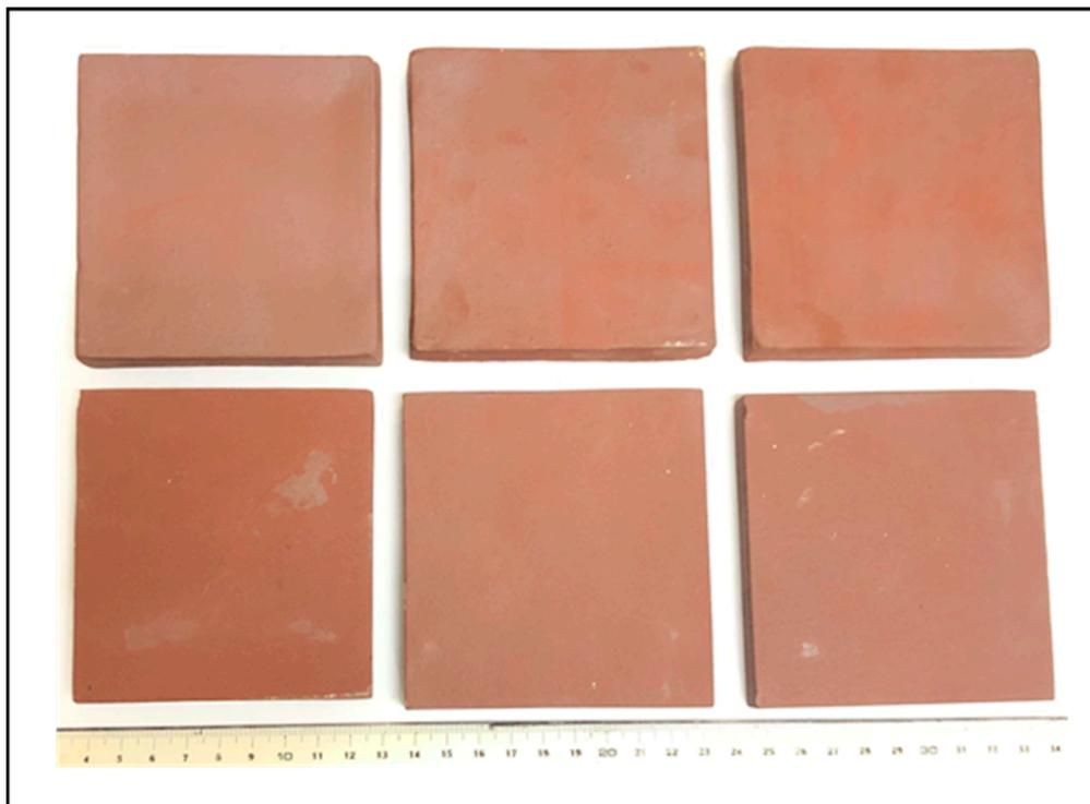
**Figure 7.** LB Tiles sintered at 1200 °C.
