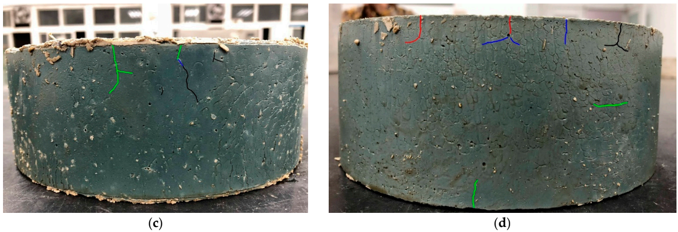
Figure 13. Effects of different polymer materials on the cracking behavior of GGBFS geopolymers. (a) Crack development in the control group. (b) Crack development with 0.7% PAM added. (c) Crack development with 0.7% SP added. (d) Crack development with 0.7% ST added. (The red, blue, green, and black lines represent the crack propagation generated after 6 h, 1 day, 2 days, and 3 days).
