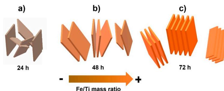
**Figure 7.** Scheme of the proposed formation mechanism of the nanosheets assembled into 3D hierarchical architectures: (a) few nanosheets appeared as house-of-cards arrangements, (b) the quantity of nanosheets seems higher and better stacked, (c) the well-organized assembly presented a book-block-like appearance with open channels.
