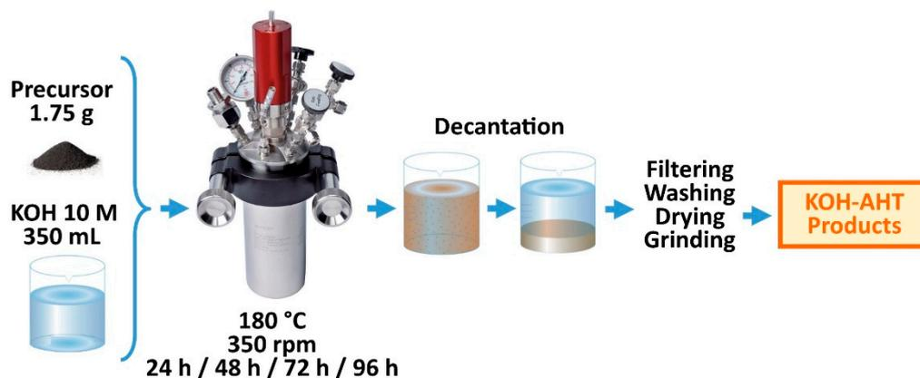
**Figure 1.** Procedure for preparation of KOH-AHT-products.
