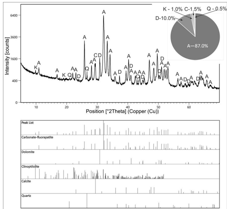
**Figure 2.** XRD pattern of a Djebel Onk sample after mechanical preparation (fraction 80–160  $\mu\text{m}$ ), with the results of qualitative analysis (table showing the matched patterns) and semi-quantitative calculations (pie chart, all values are weight). Mineral symbols: A—apatite, C—calcite, D—dolomite, K—clinoptilolite, Q—quartz.
