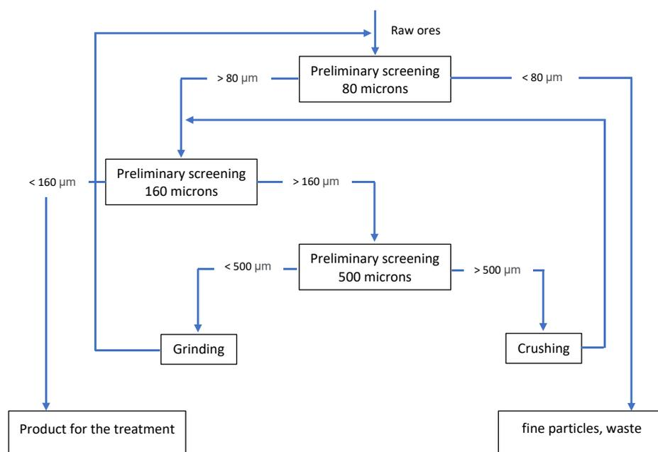
**Figure 1.** Technological procedures (mechanical preparation) conducted for preparation of 80–160 μm fraction.
