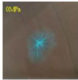
Figure 13. The crack distribution in specimen S0.
