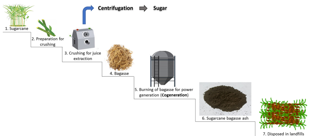
Figure 1. Steps of sugarcane bagasse ash production.
