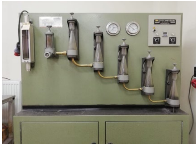
Figure 6. Cyclosizer test rig.
