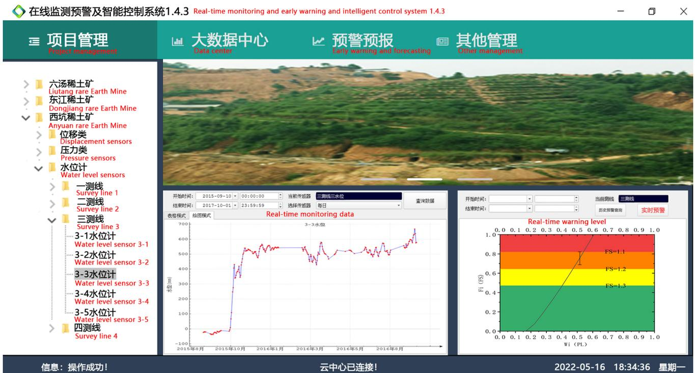
Figure 12. Self-developed landslide early warning system.
