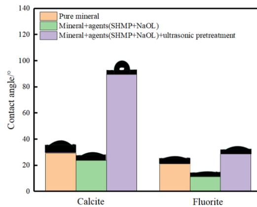
**Figure 8.** Contact angles for each treatment stage of the mineral.
