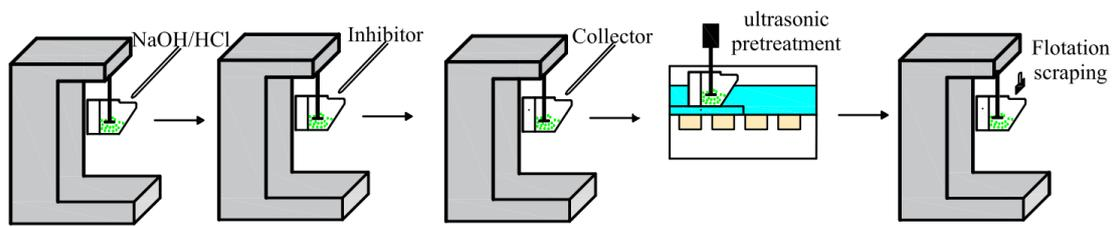
**Figure 2.** Flotation flow chart.
