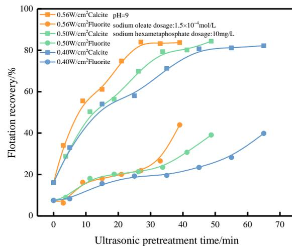
**Figure 6.** Effect of ultrasonic pretreatment time on flotation recovery.
