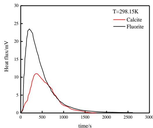
Figure 11. Adsorption heat curve.
