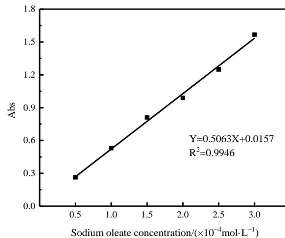
**Figure 4.** Sodium oleate concentration and absorbance label curve.
