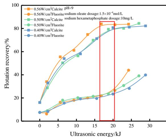
**Figure 7.** Effect of ultrasonic energy on flotation recovery.
