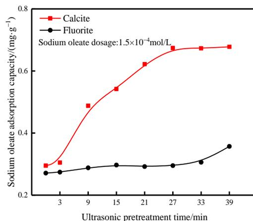
**Figure 9.** Adsorption of sodium oleate on the surface of fluorite and calcite.
