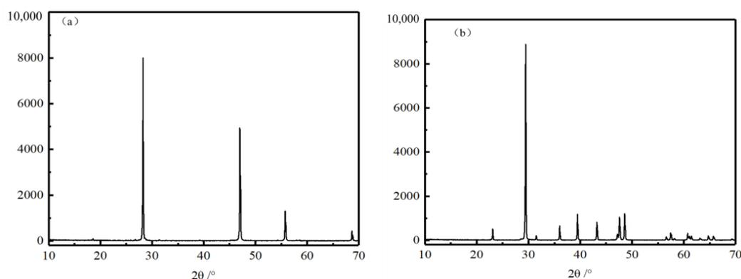
**Figure 1.** Fluorite and calcite XRD atlases. (a) Fluorite, (b) calcite.
