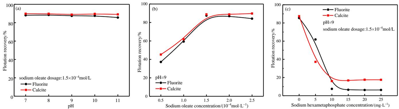
**Figure 5.** Flotation agent system. (a) pH test, (b) sodium oleate dosage test, (c) sodium hexametaphosphate dosage test.
