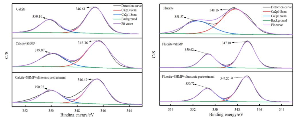
Figure 13. Fine spectral peak fitting diagram of mineral Ca2p.
