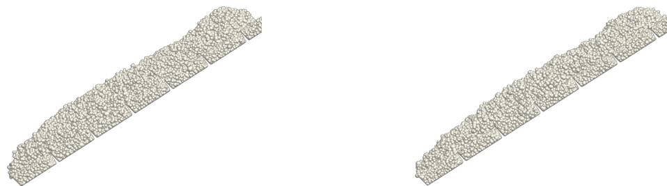
**Figure 16.** Modelled pile of fine sand (F24.7) using the JKR (left) and SJKR-A (right) models.
