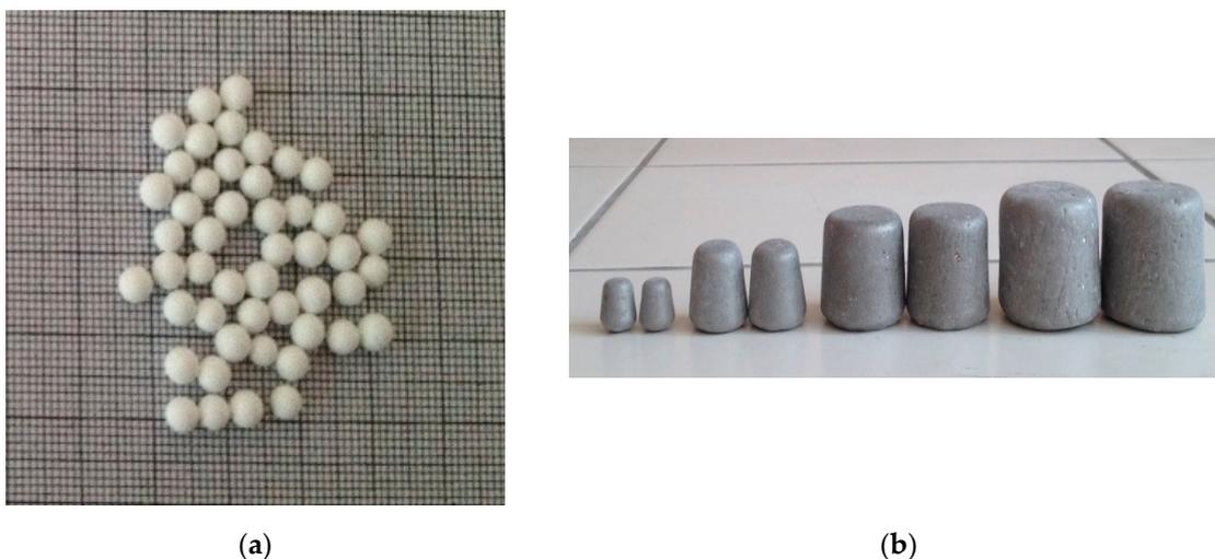
**Figure 5.** Grinding media used in this study (a) alumina balls used for stirred mill grinding, (b) cylpebs used for ball milling tests [40].
