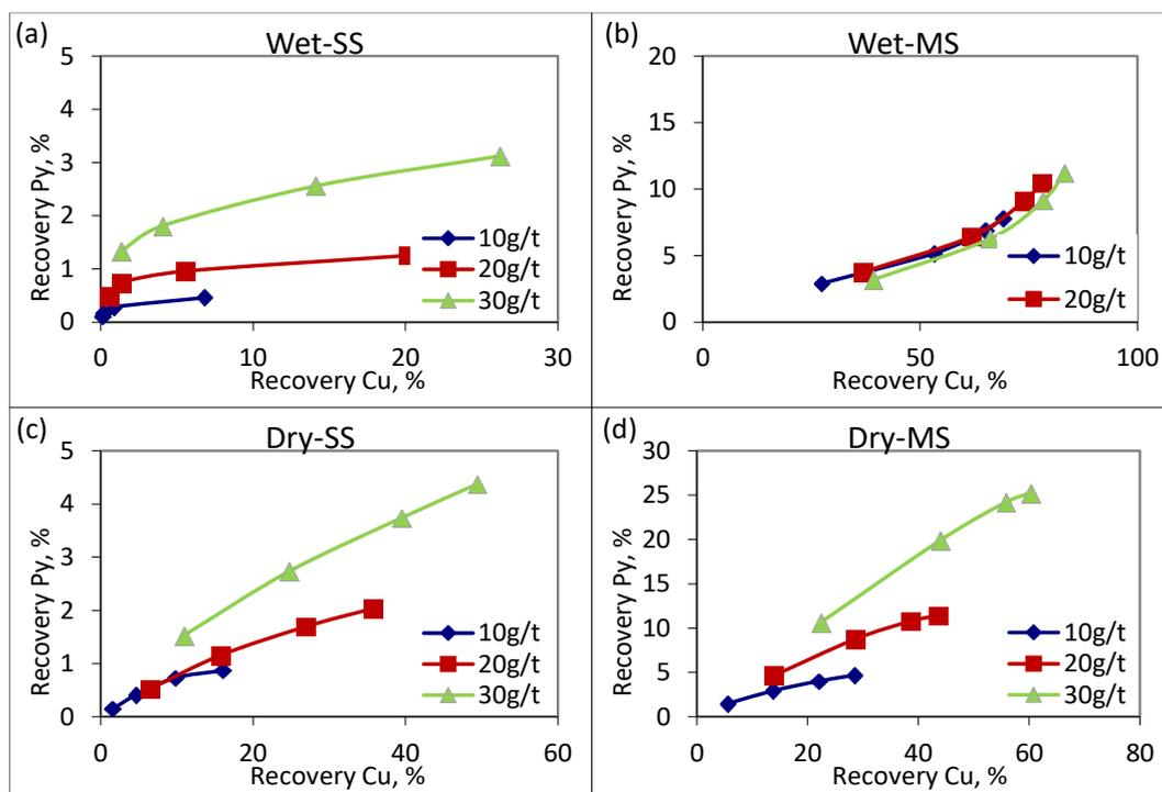
**Figure 6.** Pyrite vs. copper recovery in flotation after milling conditions of (a) Wet-SS (b) Wet-MS (c) Dry-SS (d) Dry-MS.
