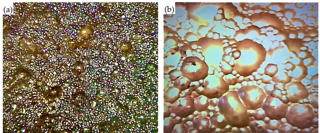
**Figure 7.** Froth images captured by Smart Froth for 30 g/t collector dosage. (a) Wet grinding with MS (b) Wet grinding with SS.
