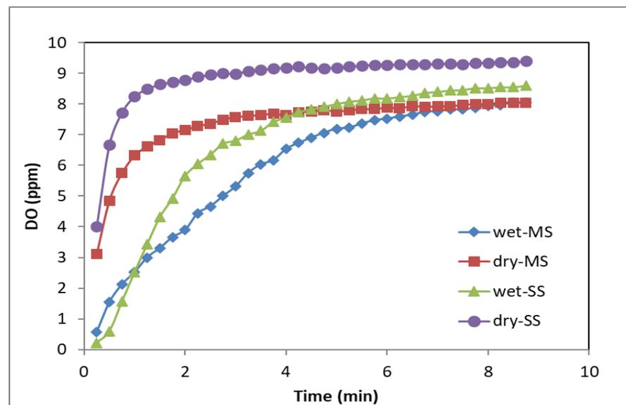
Figure 3. DO concentrations in the pulp during flotation for different milling conditions.
