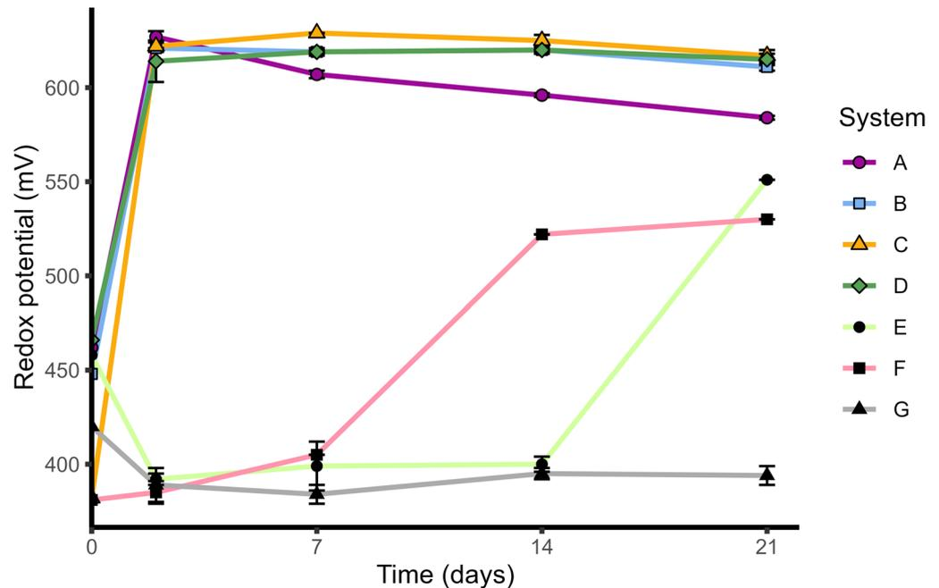
**Figure 4.** Evolution of ORP values during bioleaching tests at 30 °C with native consortium. Inoculated systems were performed in (A) distilled water, (B) MAC medium, (C) MAC medium + Fe(II) + S(0), (D) local groundwater with initial pH adjusted to 2.0. Non-inoculated controls were performed in MAC medium (E), MAC medium with Fe(II) and S(0) supplementation (F), and using a sterilized mineral with the addition of paraformaldehyde (G).
