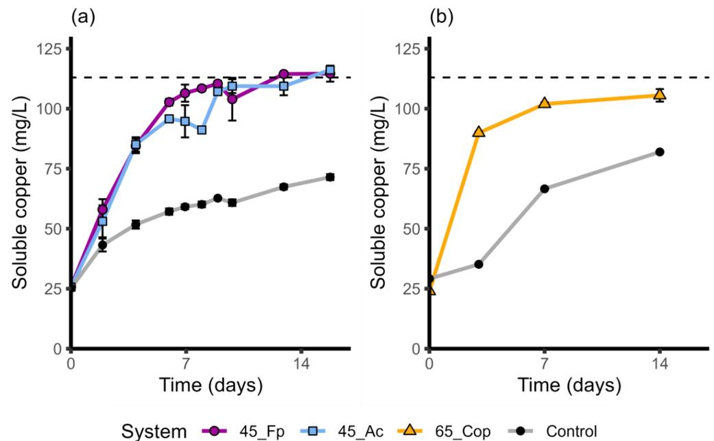
**Figure 6.** Copper recovery during bioleaching assays at 45 (a) and 65 °C (b). Sterile controls performed in MAC medium using a sterilized mineral and paraformaldehyde were included at both temperatures.
