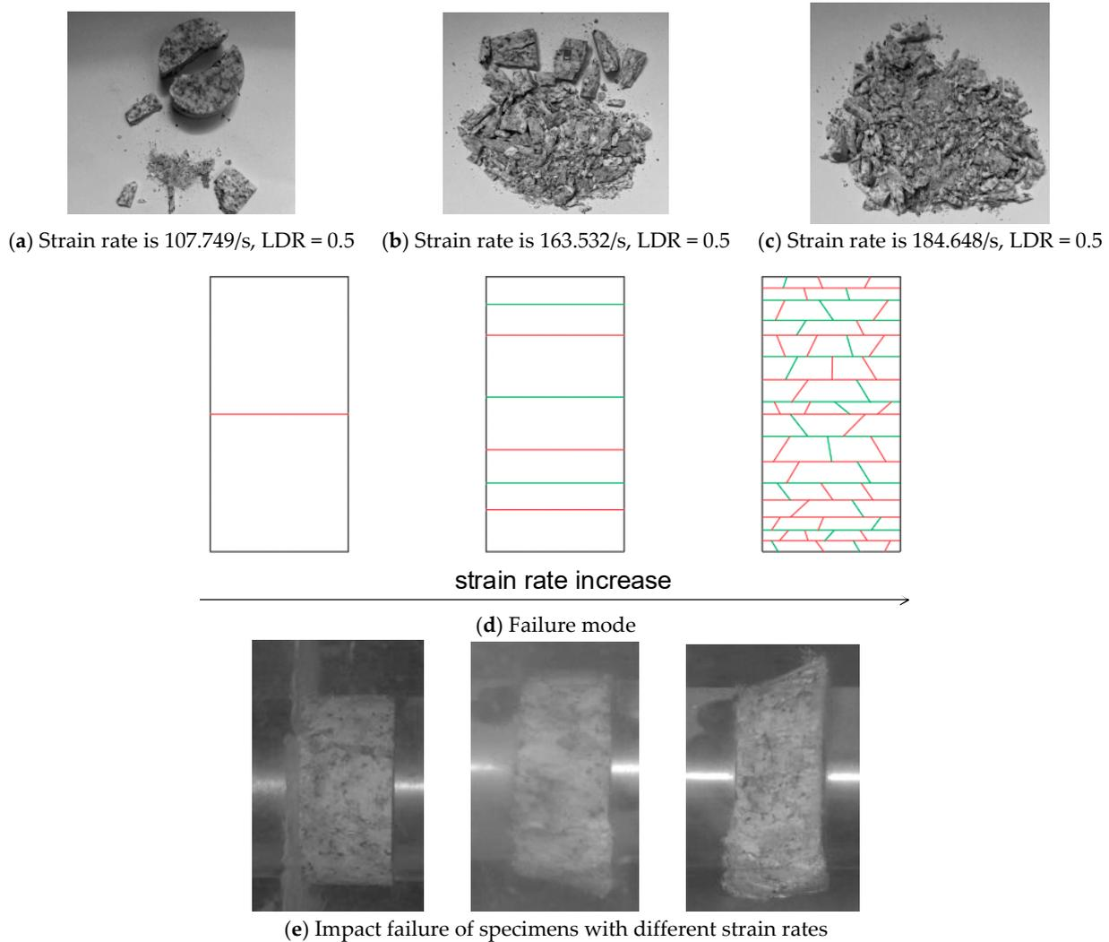
Figure 5. Influence of strain rate on specimen crushing.
