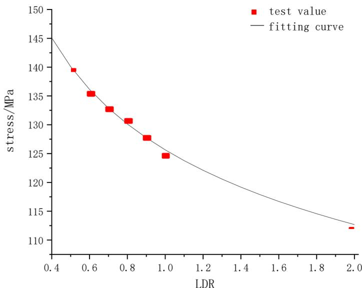
Figure 9. Size effect of rock strength under static loading.
