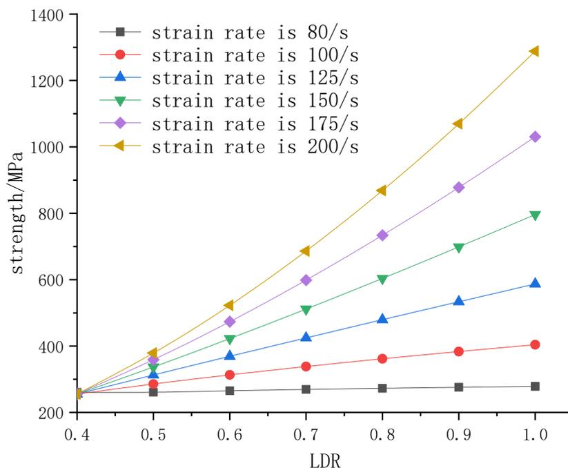
Figure 10. Size effect of dynamic rock strength.
