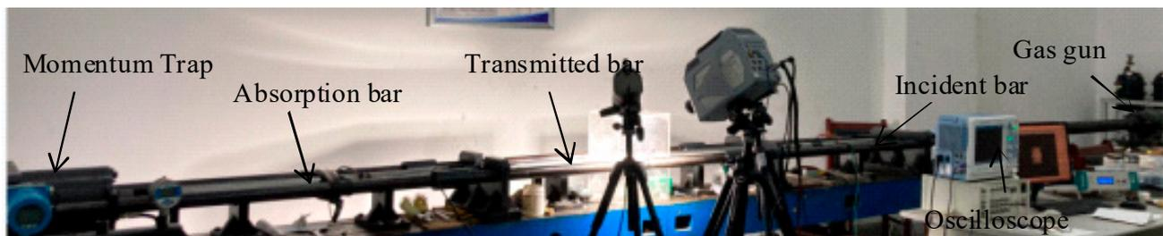
Figure 1. SHPB experimental device.
