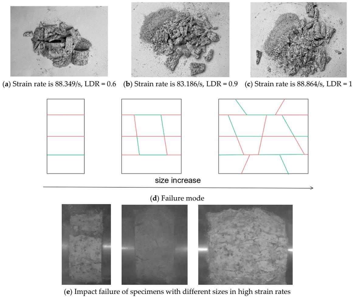
Figure 6. Influence of size on specimen crushing.
