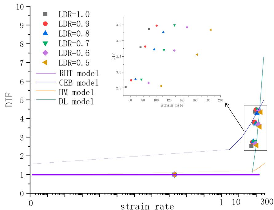
**Figure 3.** Comparison between experimental DIF values and the empirical model's values [18,21–23].
