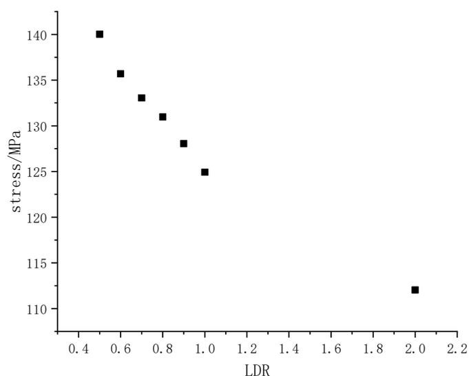
**Figure 2.** Static rock strength of different sizes.
