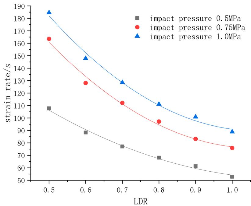
Figure 7. Relationship between strain rate and size.
