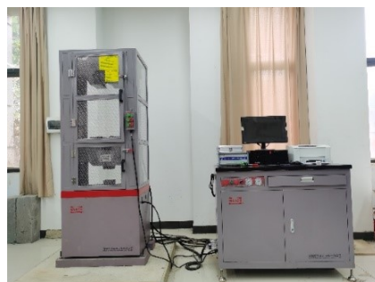
Figure 6. HUT305A type 300 kN microcomputer-controlled electrohydraulic servo universal testing machine.
