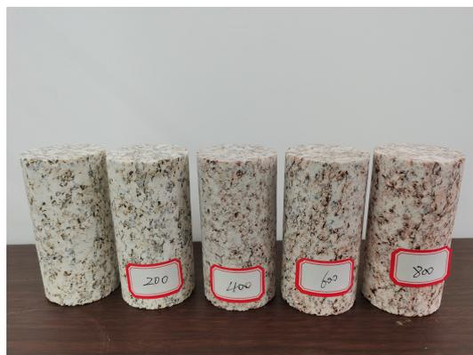
**Figure 2.** Heat-treated granite specimens.
