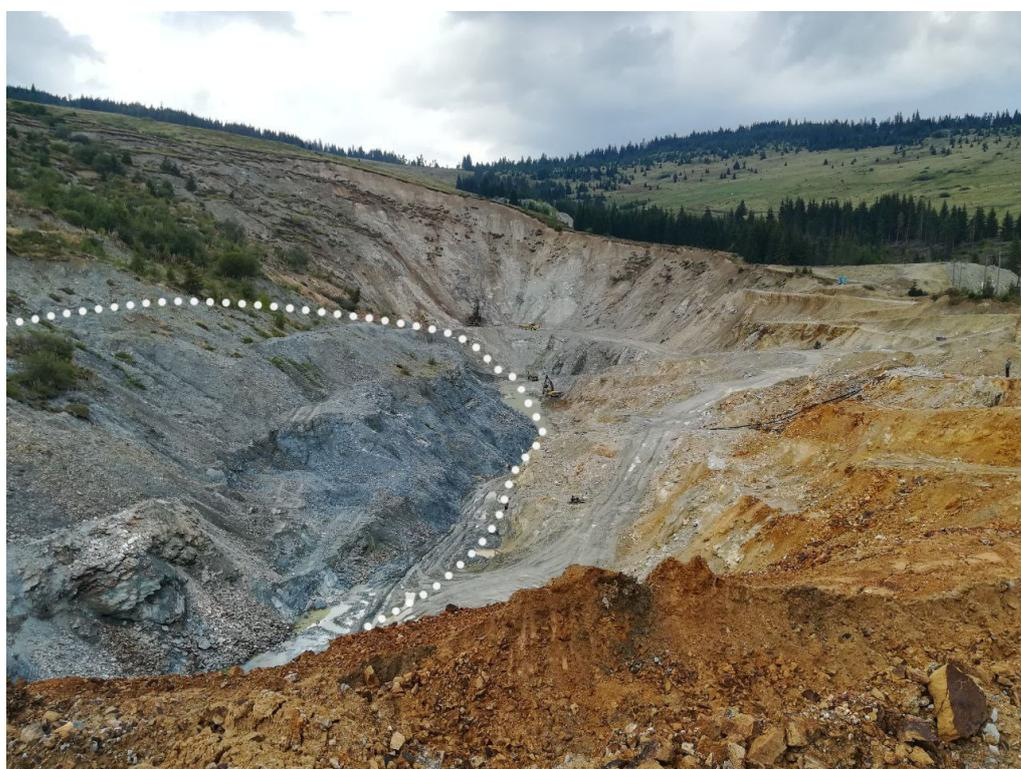
**Figure 3.** Panoramic view of the Mănăilă open pit (photo date: September 2018). The dotted line represents the mineralization presented in rhyolitic metatuffs.
