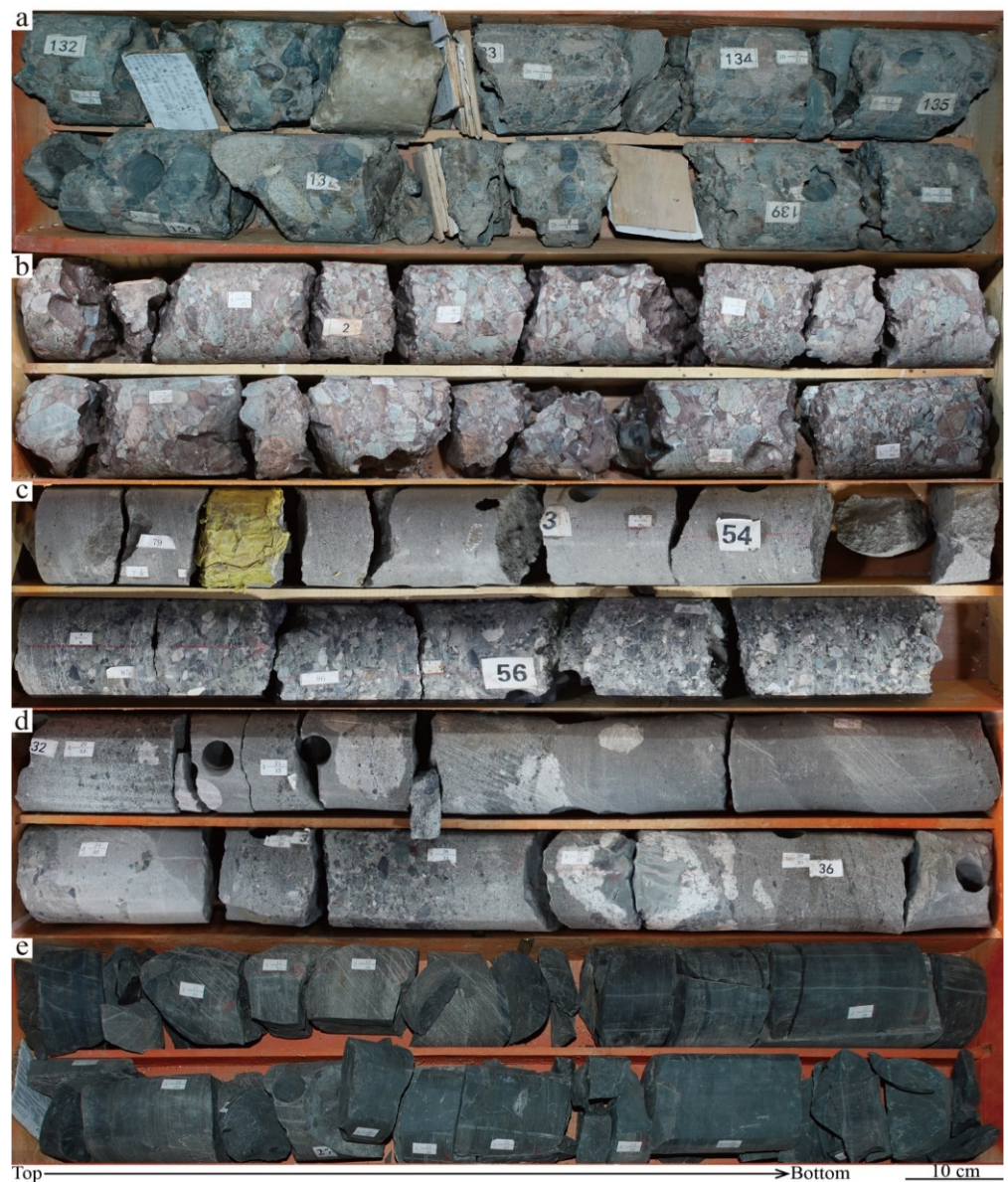
Figure 3. Core characteristics of (a) alluvial fan (JL42, 2892.52–2895.34 m), (b) fan delta plain (MH25, 3695.36–3697.36 m), (c) proximal fan delta front (J206, 4068.55–4070.44 m), (d) distal fan delta front (MH20, 4241–4242.86 m) and (e) shallow lake (JL49, 4547.84–4549.5 m) deposits.
