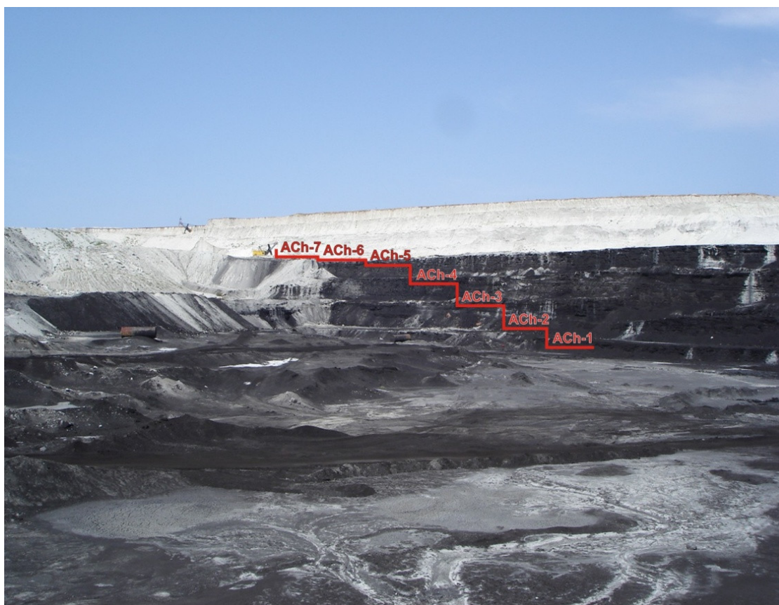
Figure 7. The sampling scheme in the Aduunchuluun coal mine (photo by Sergey Arbuzov).
