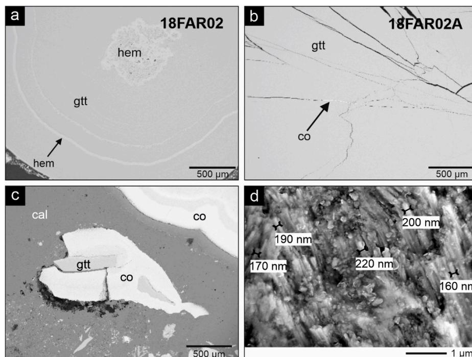
**Figure 5.** (a–c) SEM microphotographs of the most representative samples in back-scattered electron mode. (d) SEM microphotograph of botryoidal sample 18PL07. Secondary electron mode with the size of goethite crystallites (width exceeding 100 nm). Gtt = goethite; Hem = hematite; Co = coronadite group minerals; Cal = calcite.
