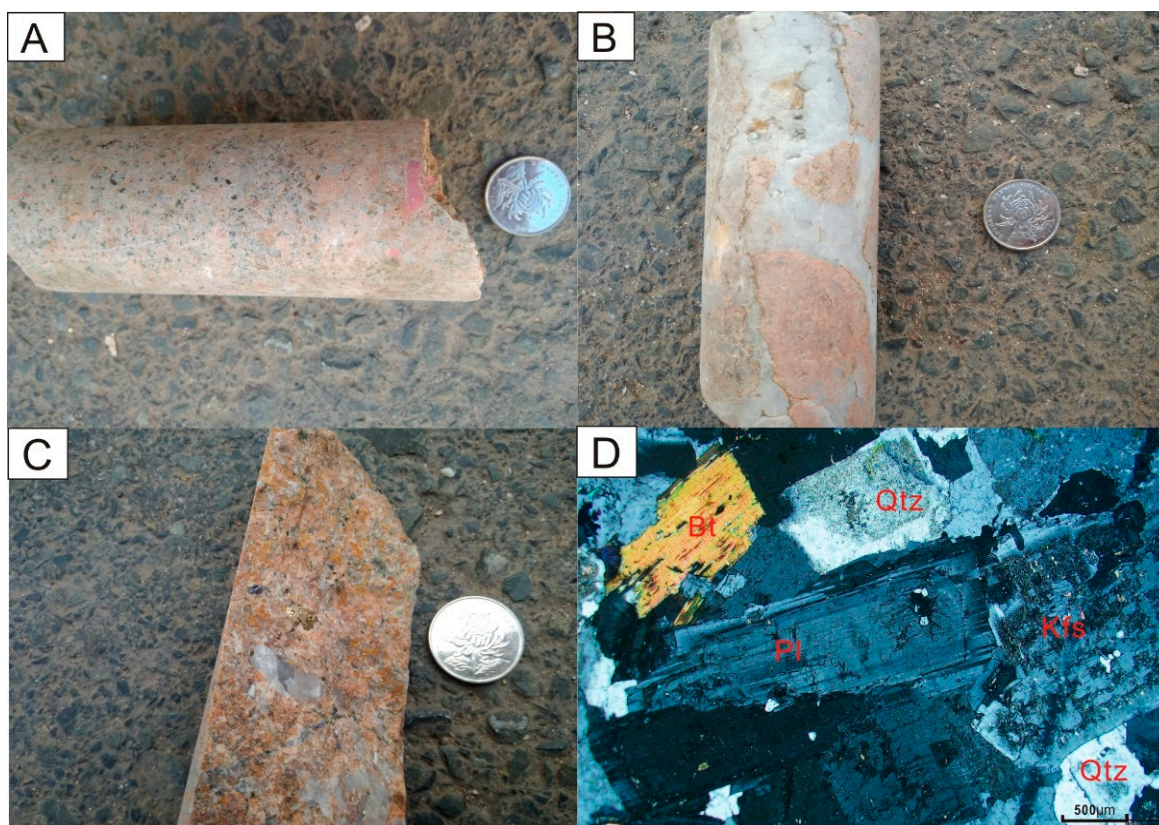
Figure 3. Microphotographs and photographs of monzogranite in the Chang'anpu area. (A) monzogranite (hand specimen); (B) brecciated monzogranite (hand specimen); (C) photomicrograph of monzogranite adjacent to the ore body; (D) photomicrograph of monzogranite (cross-polarized light). Abbreviations: Qtz—quartz; Pl—plagioclase; Bt—biotite; Kfs—potash feldspar.
