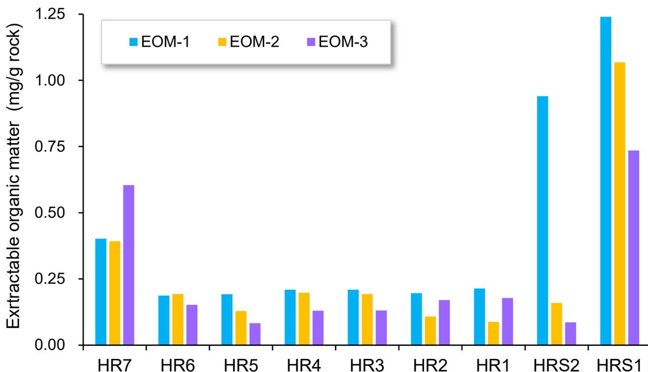
Figure 4. The amounts of extractable organic matter from sequential extraction.
