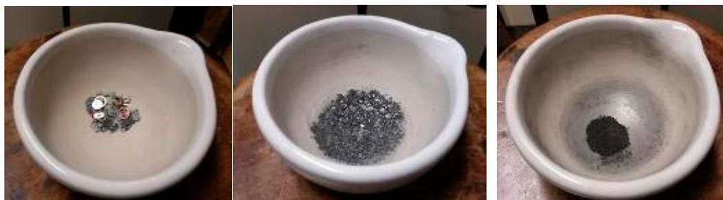
**Figure 1.** Grinding of NdFeB magnets from mobile phone devices with a mortar.
