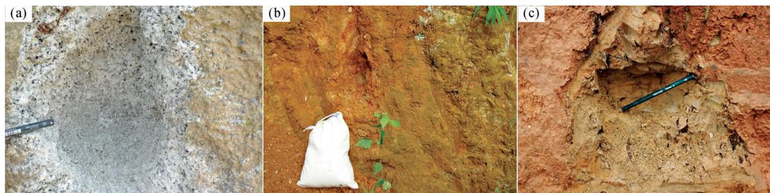
**Figure 3.** Structural characteristics of different weathering crusts: (a) Weathering crust of Zudong muscovite alkali feldspar granite in Jiangxi Province, (b) Weathering crust of Liutang rhyolite in Guangxi Province, and (c) Weathered crust of Getengzui metamorphic tuff in Jiangxi Province [15].
