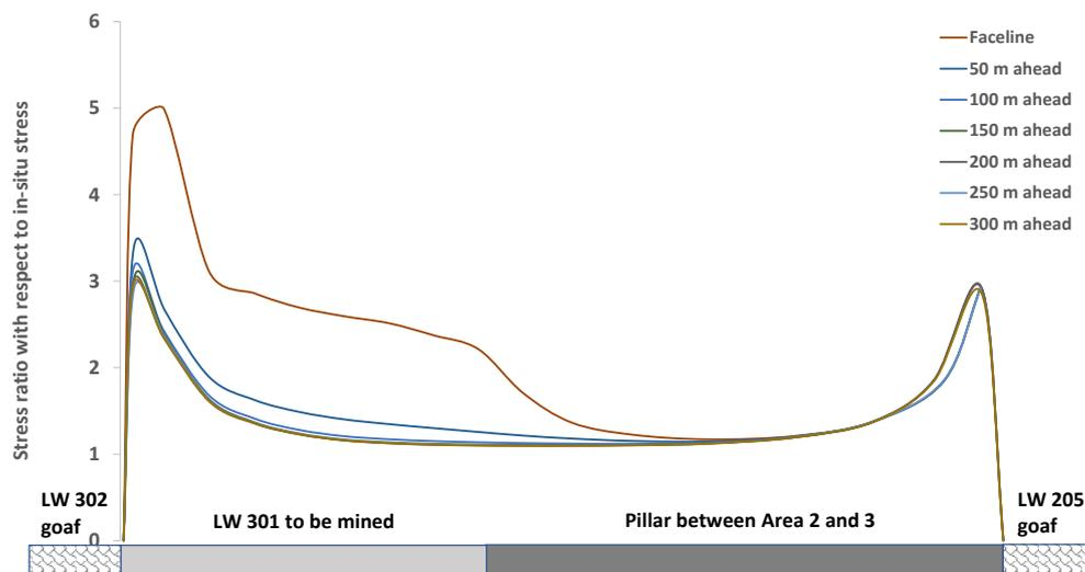
Figure 12. Vertical stress development ahead of longwall 301.
