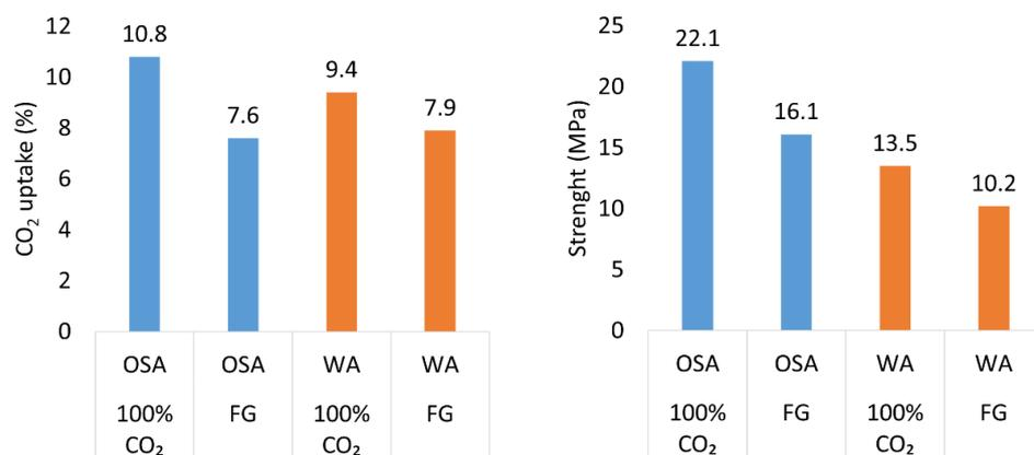
**Figure 10.** CO<sub>2</sub> uptake (left) and compressive strength (right) values at different CO<sub>2</sub> concentrations (10 bar, 25 °C, 150 kgf/cm<sup>2</sup>) (Average values obtained from min. 4 samples (std. deviation < 3%)).
