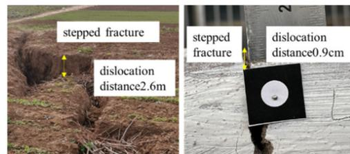
Figure 12. Comparison of field and model stepped fracture.
