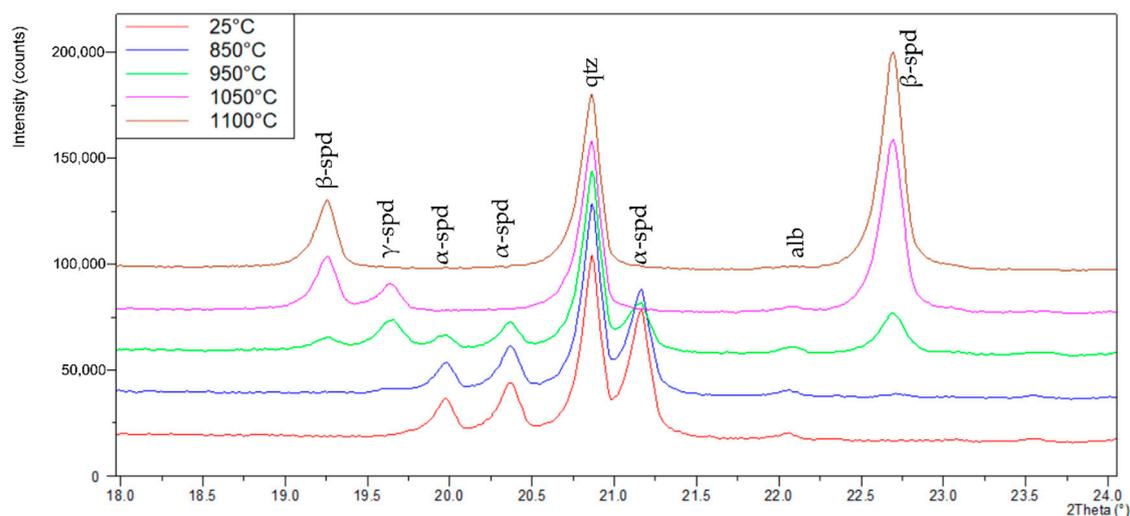
**Figure 4.** XRD diffraction patterns of the heat-treated samples compared with the reference sample at selected angles ( $18^{\circ}$  to  $24^{\circ}$   $2\theta$ ) with annotated peaks. Abbreviations: alb = albite;  $\alpha$ -spd =  $\alpha$ -spodumene;  $\beta$ -spd =  $\beta$ -spodumene;  $\gamma$ -spd =  $\gamma$ -spodumene; qtz = quartz.
