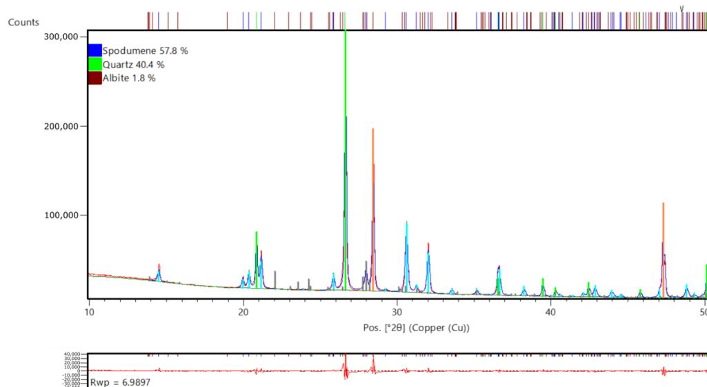
**Figure 2.** XRD diffraction pattern of non-heat-treated lithium spodumene sample. Phase quantification using the Rietveld method, zoom in to selected angle ( $10^{\circ}$  to  $50^{\circ}$   $2\theta$ ). Orange peaks belong to the silicon powder used as an internal standard. Red trace in the spectra is the observed pattern; blue trace is the calculated pattern. The red trace in the lower graphic shows the difference between the observed and calculated patterns ( $R_{wp} = 6.99\%$ ).
