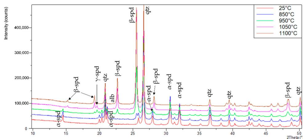
**Figure 3.** XRD diffraction patterns of the heat-treated samples compared with the reference sample at selected angles ( $10^{\circ}$  to  $50^{\circ}$   $2\theta$ ), only main peaks are annotated for clarity. Abbreviations: alb = albite;  $\alpha$ -spod =  $\alpha$ -spodumene;  $\beta$ -spod =  $\beta$ -spodumene;  $\gamma$ -spod =  $\gamma$ -spodumene; qtz = quartz.
