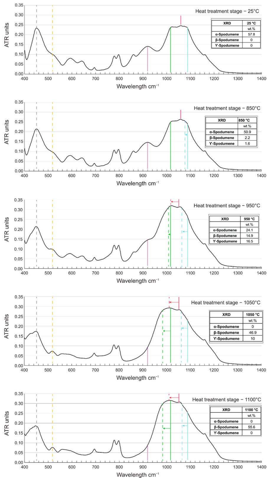
**Figure 6.** Summary of FTIR spectra through heat treatment stage, original peak maximas on the 25 °C sample indicated with solid lines.
