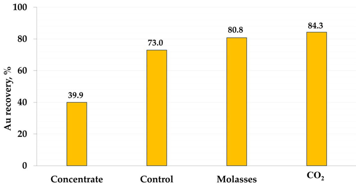
Figure 2. Gold recovery by cyanidation (%) from the concentrate as well as from the oxidation residues.
