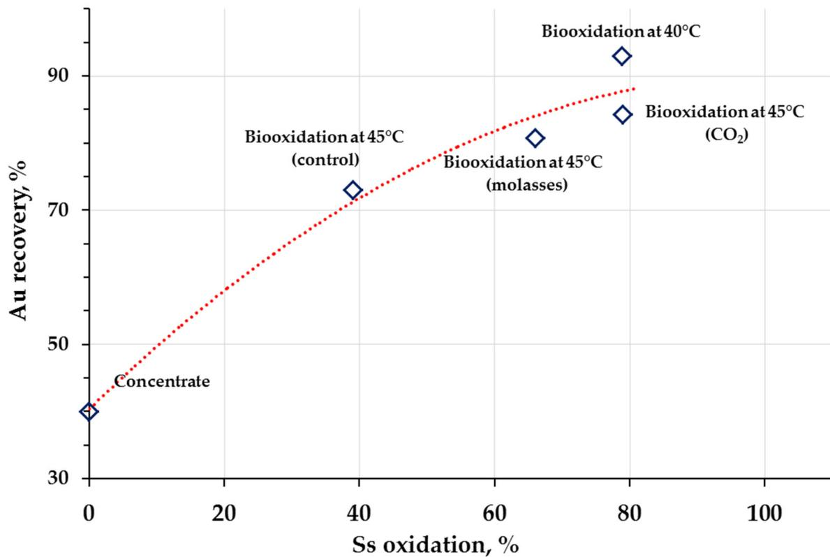
Figure 3. The dependence of gold recovery by cyanidation (%) on Ss oxidation extent.
