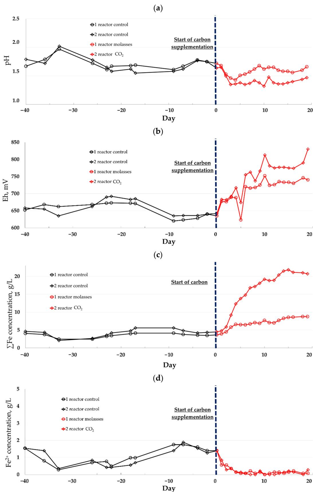
**Figure 1.** Changes in the pH (a) and Eh (b) values, total concentrations of  $Fe^{3+}$  and  $Fe^{2+}$  (c) and  $Fe^{2+}$  (d) ions (g/L) after the start of carbon supplementation.
