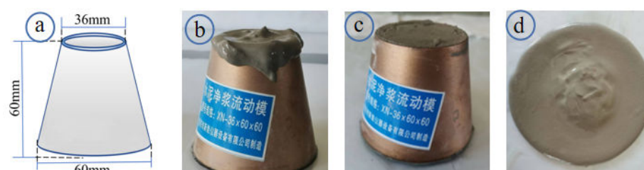
Figure 4. Paste diffusion test process: (a) prepare a slump cone with the height of 60mm and the diameter of 36 mm, 60mm, respectively; (b) grout; (c) trowl; (d) measure.
