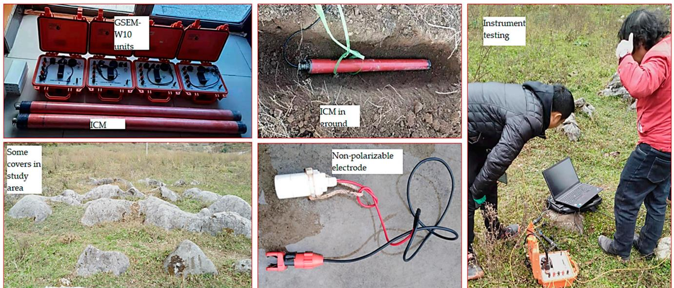
**Figure 4.** AMT field instruments used and the covers in the area. ICM: induction coil magnetometers.
